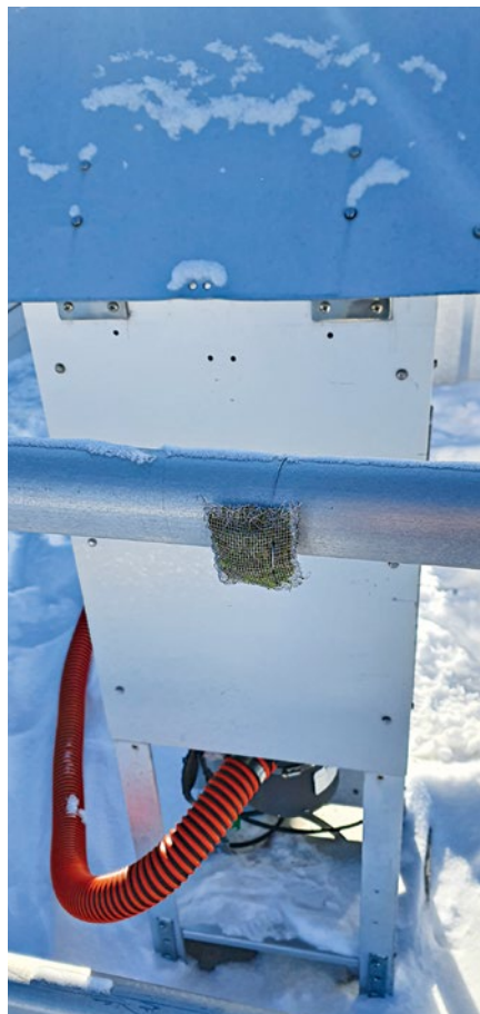
A moss bag passive air sampler for microplastics
