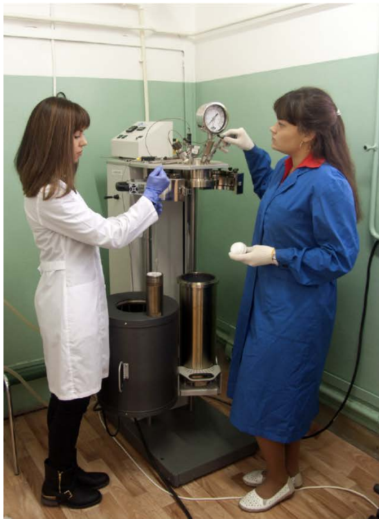
Hydrothermal synthesis (left) and general view of SIV and its exchange forms (right)
